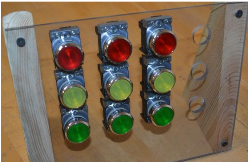
Front side of New Pushbutton Stations
