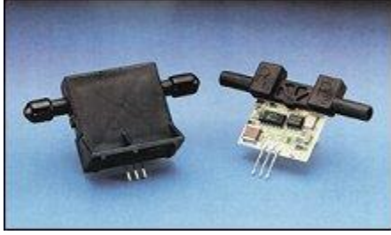
Photo 4. The output voltage of the microbridge mass air flow sensor varies in proportion to the mass flow of air or other gas through the inlet and outlet ports of the package. The packaged sensor is 1.20 in. wide by 1.24 in. long by 0.61 in. high.
