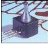
Photo 2. This totally integrated silicon pressure sensor measures 0.52 in. long by 0.44 in. wide by 0.75 in. high, including the port.
