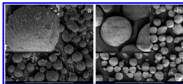
Figure 12. ESEM images of oxidized (a) C4A-950 and (b) C4A-1050 subsequent to full reduction using \text{H}_2 . Note the agglomeration in (a) caused by the complete reduction of the oxygen carrier.
