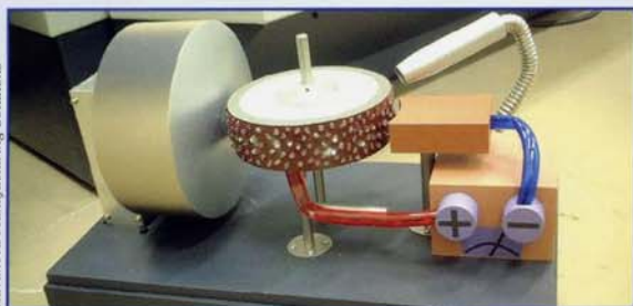
A model of an ELID grinding setup.
